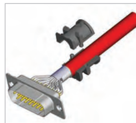
Attach the strain relief around the cable
