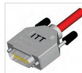
Assemble the other half (screwing force: 100-120 Ncm)
